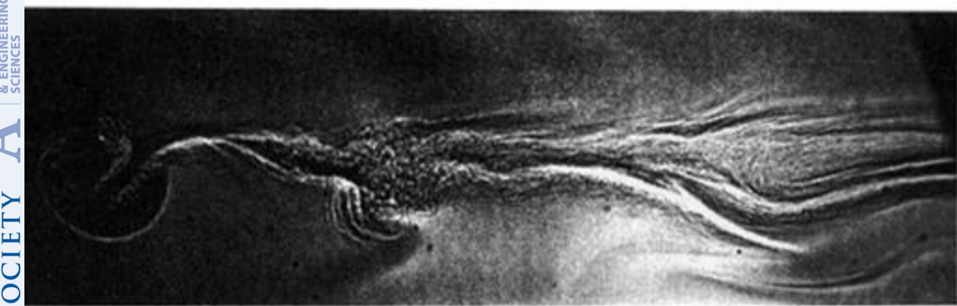
Figure 7. Type 7 flow. Same legend as figure 2, except Re = 238 , Fr = 0.73 , and \Theta = 0.94 .
