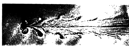
Figure 7. Type 7 flow. Same legend as figure 2, except Re = 238 , Fr = 0.73 , and \Theta = 0.94 .
